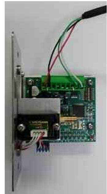
Fig 3a. Basic Assembly with close up of wall sensor connections.
