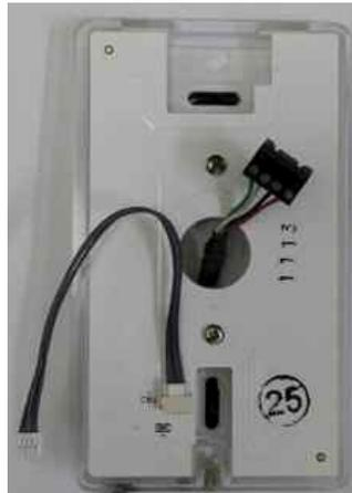
Fig 2. Route interface cable through center hold at display enclosure backplate.
