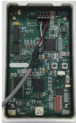
Fig 3. Interface connected to 4-pin header at top of display module.
